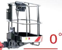
The SPS system is what allows the use of the Billennium Spiderbooms even without lowering the stabilizers, levelling longitudinally up to a maximum of 10° with a maximum working height of 8,6 m.
