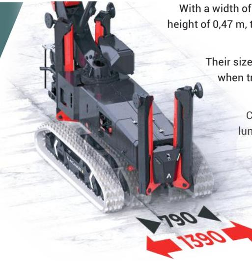
The track tensioning system is a hydraulic cylinder directly connected to and controlled by the main hydraulic system.
